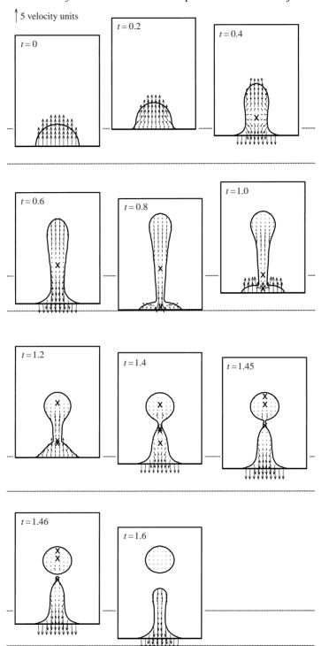
Figure 6. The droplet ejection process without the formation of a crater. Time is in periods. Velocity vectors are shown in every third cell. The horizontal lines indicate the minimum and maximum displacement of the base. Stagnation points are indicated by  $\times$ . Re=10, Bo=0, A=25,  $\Omega=1$ ,  $\theta=0$ ,  $\alpha=0.001$ , and  $\beta=0.001$ . The arrow at top left shows the velocity scale in dimensionless units.  $30\times80$  grid cells in half of the domain shown.
