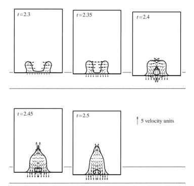
FIGURE 12. The bubble entrapment process. Time is in periods. Velocity vectors are shown in every third cell. The horizontal lines indicate the minimum and maximum displacement of the base.  $Re=10,\ Bo=0,\ A=20,\ \Omega=1,\ \theta=0,\ \alpha=0.001,\ \text{and}\ \beta=0.001.\ 30\times80$  grid cells in half of domain shown.
