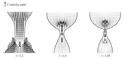
FIGURE 7. Close-up of pinch-off. Time is in periods. Velocity vectors are shown in every cell. Stagnation points are indicated by  $\times$ . Re=10, Bo=0, A=25,  $\Omega=1$ ,  $\theta=0$ ,  $\alpha=0.001$ , and  $\beta=0.001$ .  $30\times80$  grid cells.
