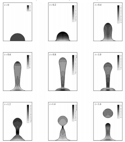
FIGURE 8. Pressure contours in the droplet ejection process without the formation of a crater. Time is in periods. Re = 10, Bo = 0, A = 25,  $\Omega = 1$ ,  $\theta = 0$ ,  $\alpha = 0.001$ , and  $\beta = 0.001$ .  $30 \times 80$  grid cells in half of domain shown.
