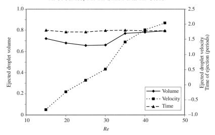
FIGURE 15. The effect of the Reynolds number on the response.  $Bo=0, A=20, \Omega=1, \theta=0,$   $\alpha=0.001, \text{ and } \beta=0.001.$
