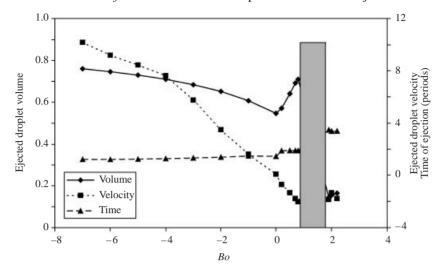
FIGURE 14. The effect of the Bond number on the response. Re=10, A=25,  $\Omega=1$ ,  $\theta=0$ ,  $\alpha=0.001$ , and  $\beta=0.001$ . Ejection does not occur in the amplitude range delineated by the grey bar.
