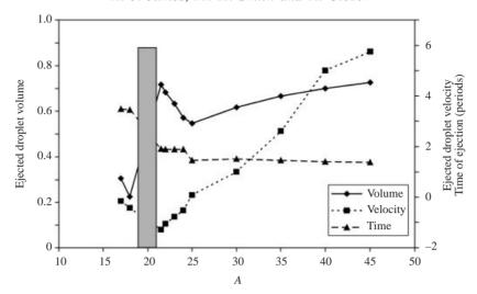
FIGURE 13. The effect of the forcing amplitude on the response. Re = 10, Bo = 0,  $\Omega = 1$ ,  $\theta = 0$ ,  $\alpha = 0.001$ , and  $\beta = 0.001$ . Ejection does not occur in the amplitude range delineated by the grey bar.
