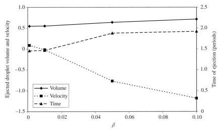
FIGURE 19. The effect of the viscosity ratio on the response. Re = 10, Bo = 0, A = 25,  $\Omega = 1$ ,  $\theta = 0$ , and  $\alpha = 0.001$ .
