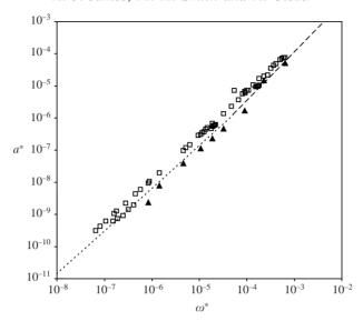
FIGURE 20. The droplet ejection threshold. Filled symbols: present simulations. Open symbols: experimental data of Range *et al.* Dotted line: low-viscosity correlation of Goodridge *et al.* Dashed line: high-viscosity correlation of Goodridge *et al.*
