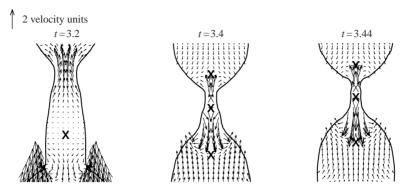
FIGURE 10. Close-up of pinch-off. Time is in periods. Velocity vectors are shown in every cell. Stagnation points are indicated by  $\times$ . Re = 10, Bo = 0, A = 18,  $\Omega = 1$ ,  $\theta = 0$ ,  $\alpha = 0.001$ , and  $\beta = 0.001$ .  $30 \times 80$  grid cells.
