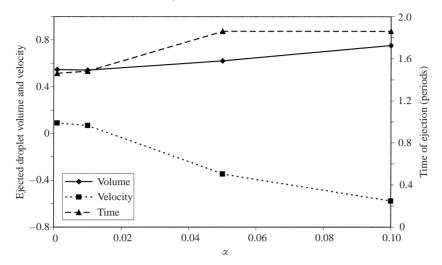
FIGURE 18. The effect of the density ratio on the response. Re = 10, Bo = 0, A = 25,  $\Omega = 1$ ,  $\theta = 0$ , and  $\beta = 0.001$ .
