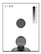
FIGURE 11. Pressure contours in the droplet ejection process with the formation of a crater. Time is in periods. Re = 10, Bo = 0, A = 18,  $\Omega = 1$ ,  $\theta = 0$ ,  $\alpha = 0.001$ , and  $\beta = 0.001$ .  $30 \times 80$  grid cells in half of domain shown.
