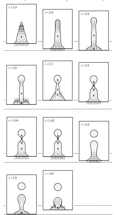
FIGURE 9. The droplet ejection process with the formation of a crater. Time is in periods. Velocity vectors are shown in every third cell. The horizontal lines indicate the minimum and maximum displacement of the base. Stagnation points are indicated by  $\times$ . Re=10, Bo=0, A=18,  $\Omega=1$ ,  $\theta=0$ ,  $\alpha=0.001$ , and  $\beta=0.001$ .  $30\times80$  grid cells in half of the domain shown.
