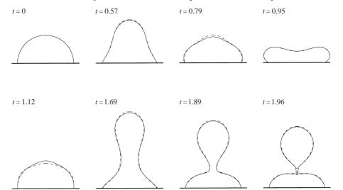
FIGURE 4. Drop shape profile evolution. Time in periods. Re = 22.6, Bo = 0,  $\Omega = 0.81$ , A = 5.61,  $\alpha = 0.001$ ,  $\beta = 0$ . Solid line: present work; dashed line: Wilkes & Basaran (2001).
